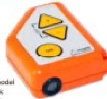
**EC II Clinometer** Art no 15-102-1011 Specify model on order as Feet/Degrees; Feet/Percent; Meter/Degrees; Meter/Percent. Delivered with lanyard and instructions.
